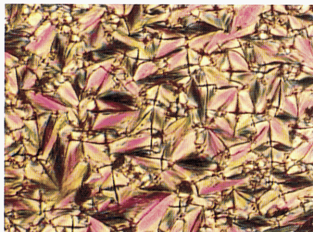
Figure 7. Optical fan-shaped texture observed for the smectic phase of poly(1b).
